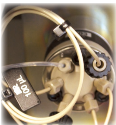
Exchangeable Sample Loop made of PEEK
